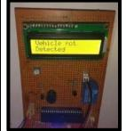
Step 6: IR sensor will detect the vehicle is parked or not.
